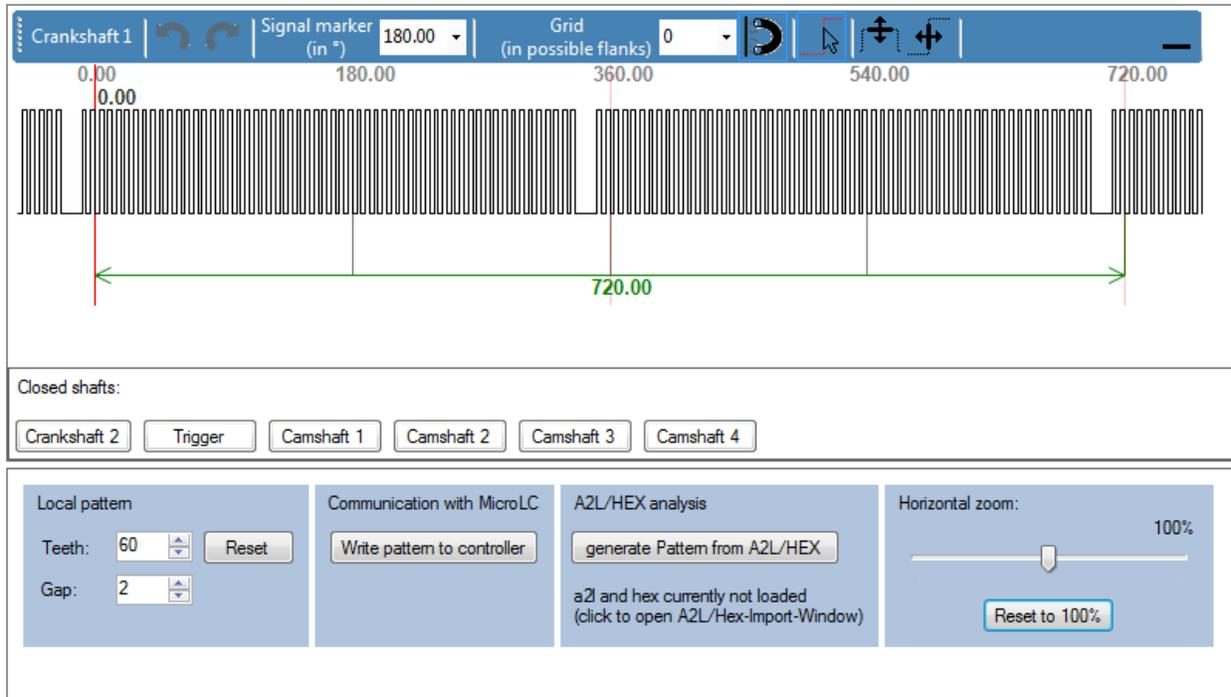
Figure 3: MicroLC Software - Illustration of crankshaft signal
