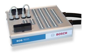
The Breakout Box BOB enables the operator to perform measurements and modify connections during operation. The jumpers allow to individually open or close each single connection without removing the jumper. Jacks provide access to all signals for measurement purposes. The box is essential for development and test environments in the lab and vehicle.
